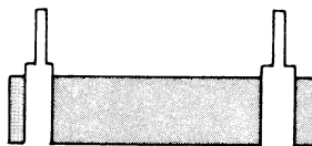
(b) Example of (+) synchronizing signal
